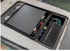
Build in Motor controller IP 67
